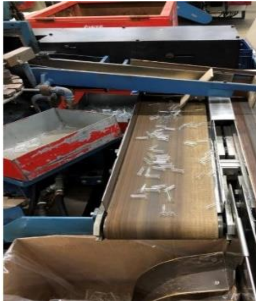
Figure 12 Movable plate removal belt from the tempering furnace
